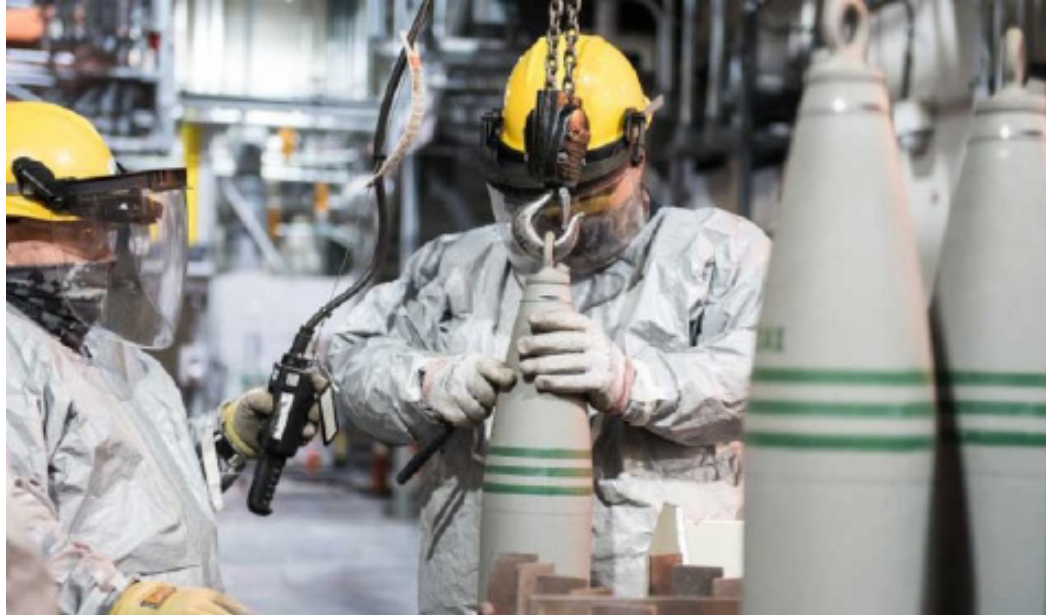
Army specialists at the USA's Blue Grass Chemical Agent Destruction Plant disassembling 155mm shells.
